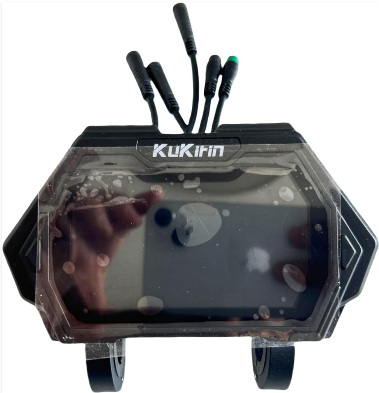
Figure 2.1: Front view of the Elekirin TFM13-FEIMI-11 Version B LCD display. This image shows the main screen and the "KuKirin" branding at the top, along with the various cable connections extending from the top of the unit.
