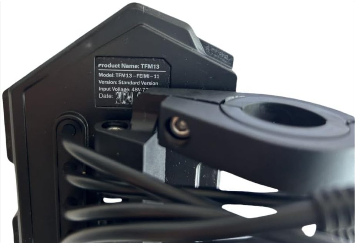
Figure 2.2: Close-up of the product label. This label confirms the product name "TFM13", model "TFM13-FEIMI-11", and specifies the input voltage range of 48V-72V.
