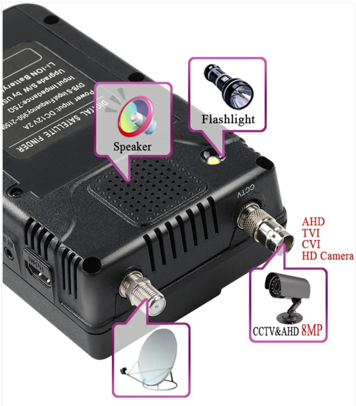
Image: Side view of the satellite finder, highlighting the built-in speaker, flashlight, BNC connector for AHD/TVI/CVI HD cameras, and F-type connector for satellite dish input.
