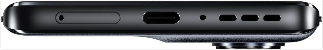
Image: Bottom view of the Motorola Edge 5G (2024), highlighting the SIM card slot and USB-C port.
