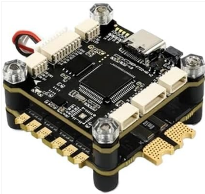
Image 1: The GEP-F722-HD V2 Flight Controller and 50A 4in1 ESC Stack. This image displays the compact design of the stack, highlighting the flight controller mounted atop the 4-in-1 ESC, with various connection pads visible.
