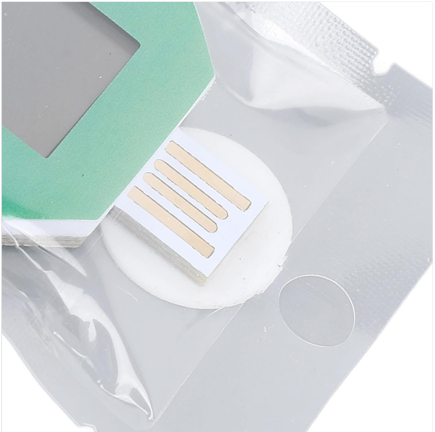
Figure 4.1: A detailed view of the USB connector, which is integrated into the data logger's design for direct connection to a computer.
