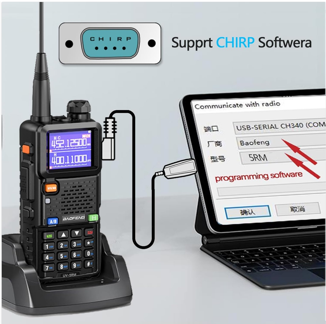
Image 3.2: The UV-5RM connected to a computer for programming using CHIRP software.
