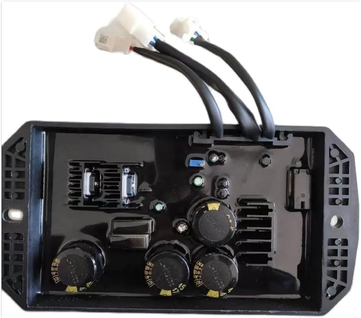
Figure 2.1: Top view of the LIHUA AVR TT91-1, showing the main circuit board, capacitors, heat sinks, and the attached 8-wire harness with connectors.
