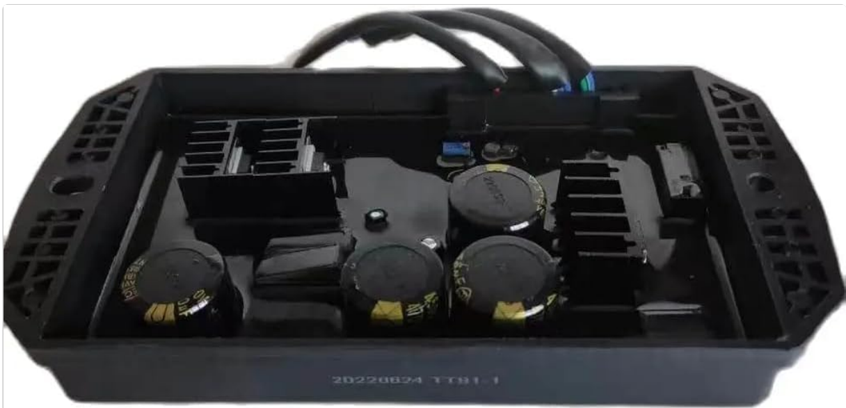
Figure 2.2: Side view of the AVR unit, displaying the manufacturing date and the model number "TT91-1" printed on the casing.
