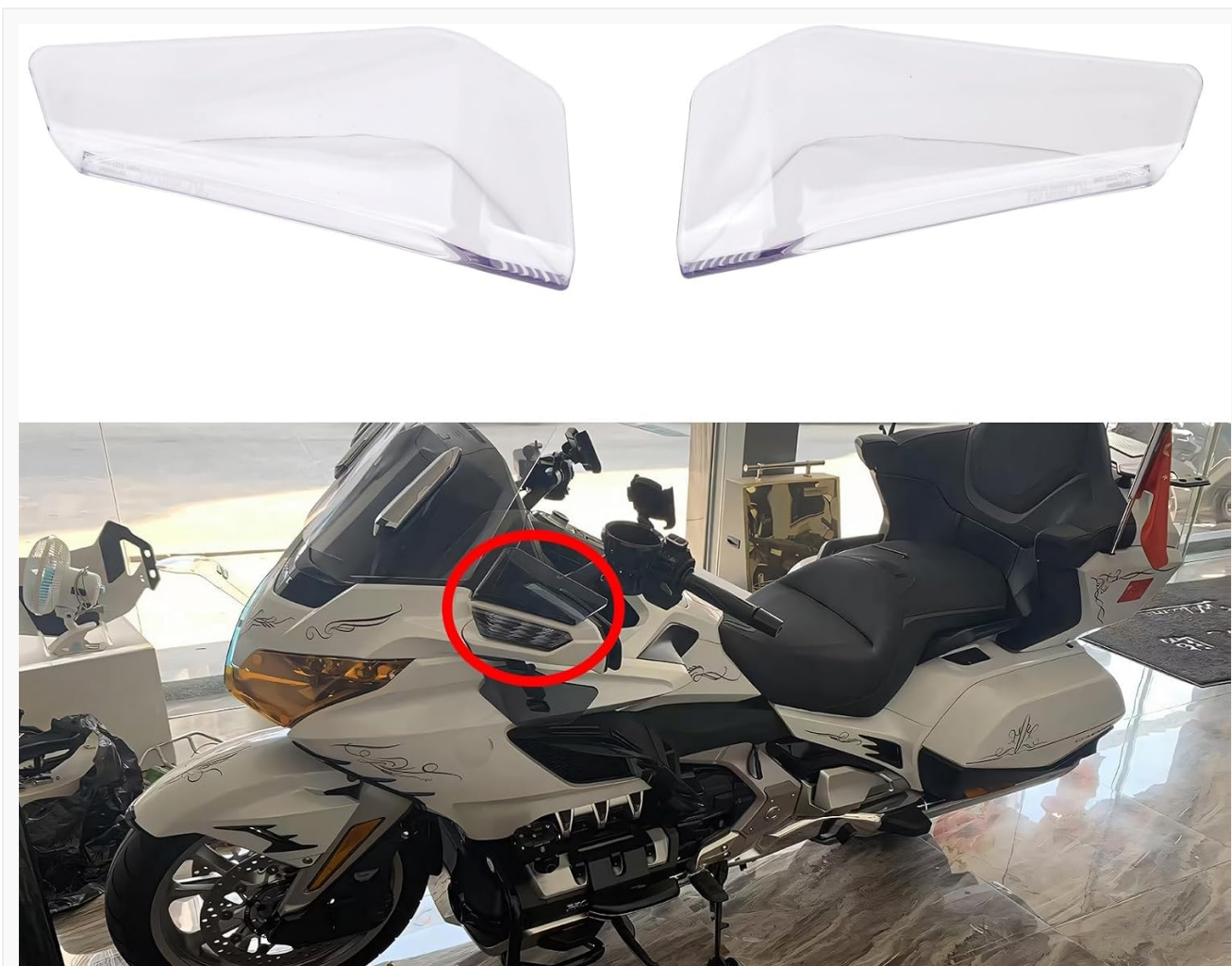
Figure 3: Installation Location. The accessories are installed on the fairing near the rearview mirrors of the Honda GoldWing.
