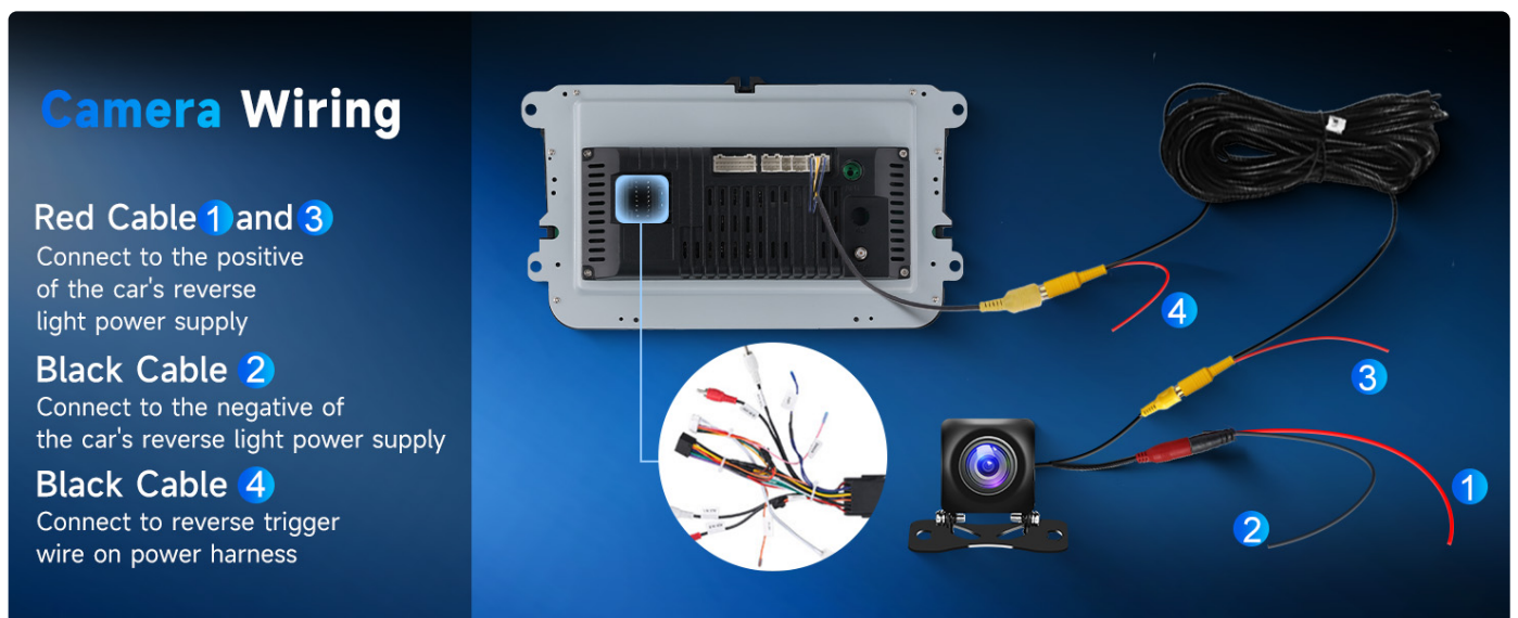
Image 3.6: Backup camera wiring diagram.
