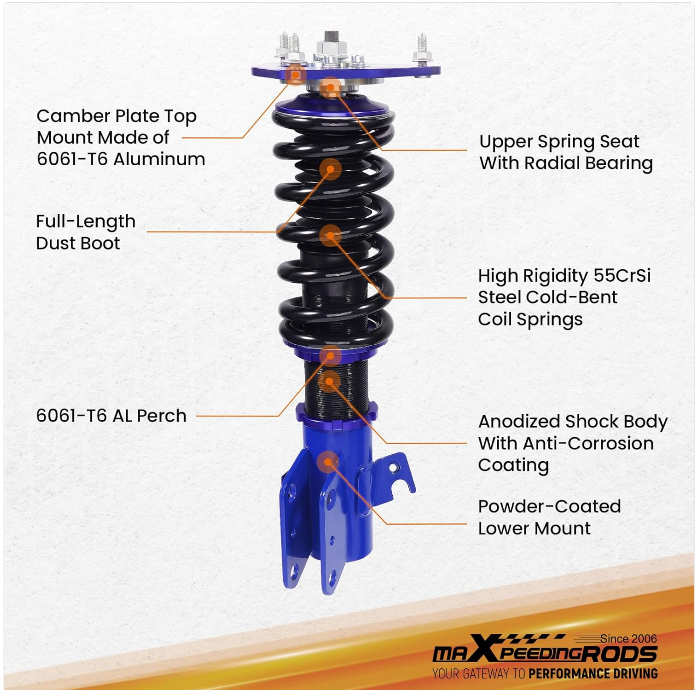
Image 4.1: Detailed component breakdown of a maxpeedingrods coilover, highlighting the Camber Plate Top Mount (6061-T6 Aluminum), Upper Spring Seat with Radial Bearing, Full-Length Dust Boot, High Rigidity 55CrSi Steel Cold-Bent Coil Springs, 6061-T6 AL Perch, Anodized Shock Body with Anti-Corrosion Coating, and Powder-Coated Lower Mount.
