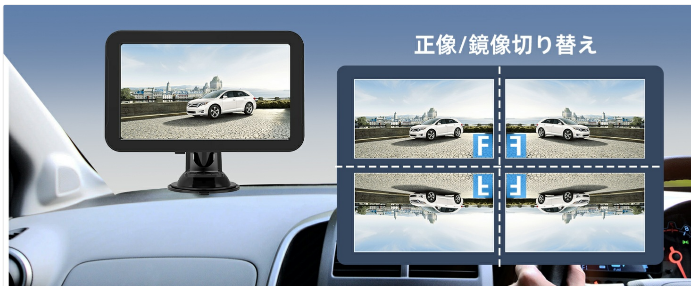
Image 4.1: Illustration of normal and mirror image display options.
