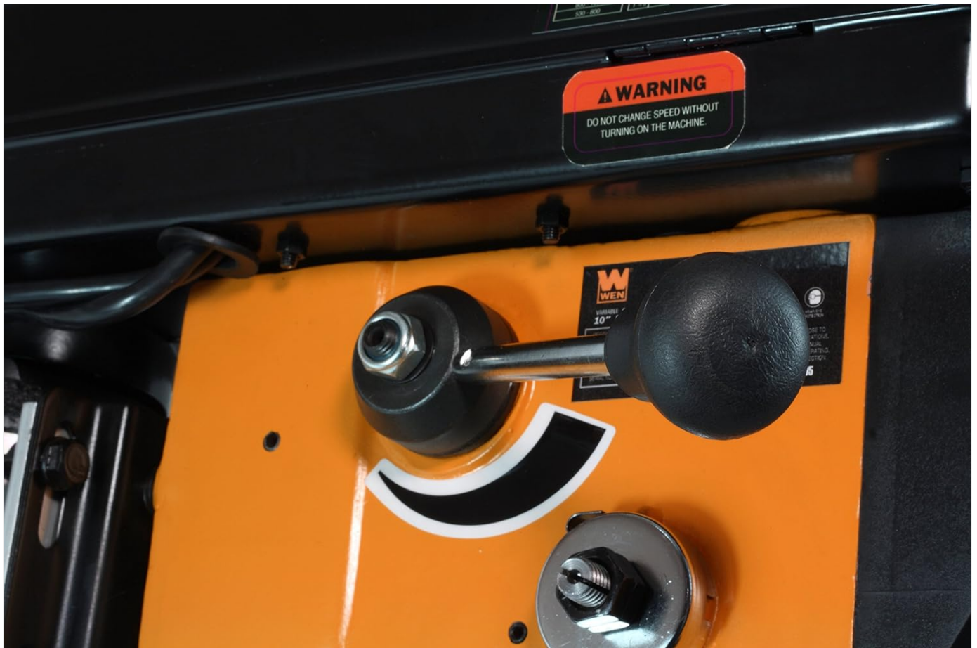
Figure 4.2: The lever for mechanical variable speed adjustment.
