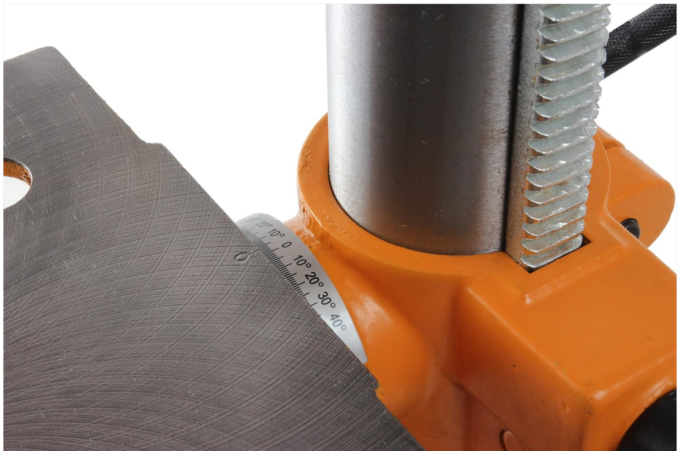
Figure 4.3: Worktable with angle markings for precise bevel drilling.
