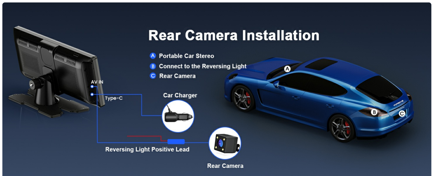
Figure 2.5: Rear Camera Installation Diagram
