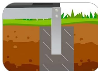
Figure 5.2.2: Greenhouse Dimensions and Anchoring. This image shows the overall dimensions of the greenhouse (12'4" wide, 6' high at eaves, 6'5" door height) and highlights options for securing the greenhouse against wind, either by fixing it to a board (using LD07) or mounting it into concrete (using BJ05). Proper anchoring is essential for stability.
