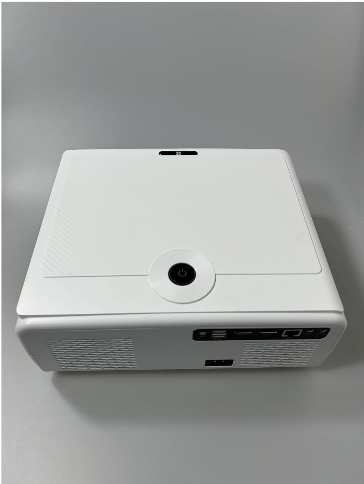
Figure 4.3: Rear View. This image illustrates the rear panel of the Henhoor H6 projector, where various input and output ports are located, including HDMI, USB, and audio jacks.
