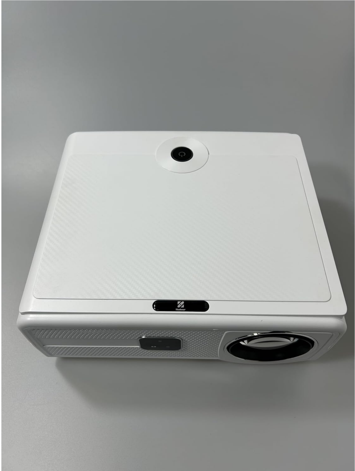
Figure 4.1: Top View. This image displays the top surface of the Henhoor H6 projector, featuring the central power button and the sliding lens cover mechanism. The textured surface is also visible.
