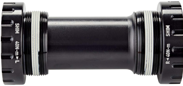
Figure 2: Side view of the Praxis BSA 68/73mm Bottom Bracket, highlighting the "SHIM" and torque specifications (40N-m) on the cups.
