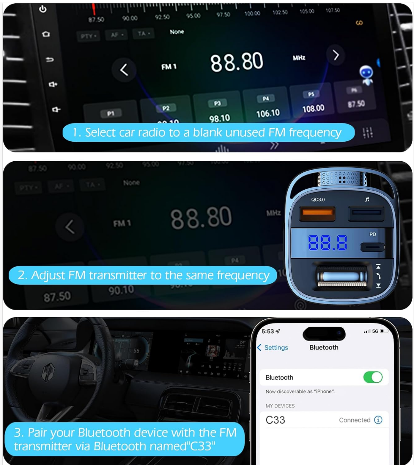
Image 4.1: Visual guide for setting up the LIHAN C33. This image illustrates the three main setup steps: 1. Selecting a blank FM frequency on the car radio (e.g., 88.80 MHz). 2. Adjusting the FM transmitter to the same frequency. 3. Pairing your Bluetooth device with the transmitter, which appears as 'C33' in your phone's Bluetooth settings.
