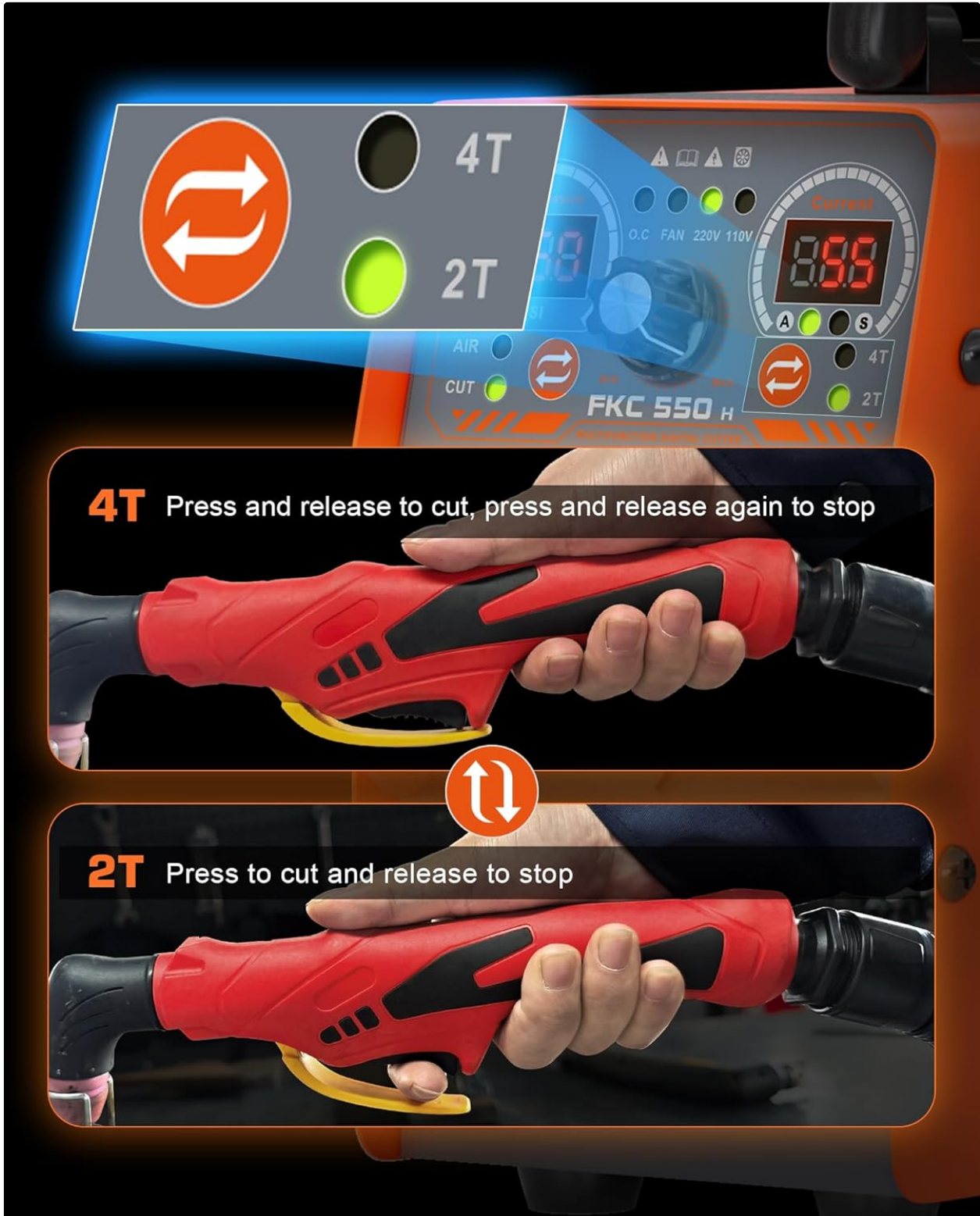
Image 5.2: Illustration of the 2T and 4T torch trigger operation for different cutting scenarios.
