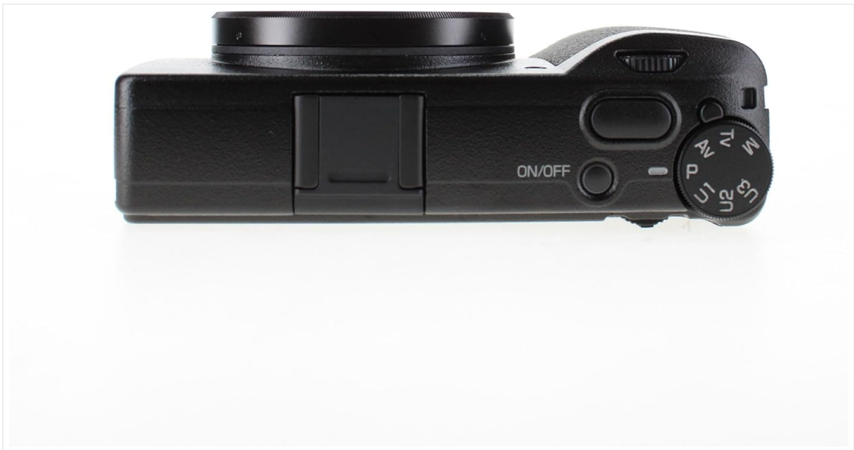
Figure 3: Top View. This view illustrates the top panel of the camera, featuring the ON/OFF button, Shutter button, and a mode dial with settings such as Program (P), Aperture Priority (Av), Shutter Priority (Tv), Manual (M), and three User-defined modes (U1, U2, U3).
