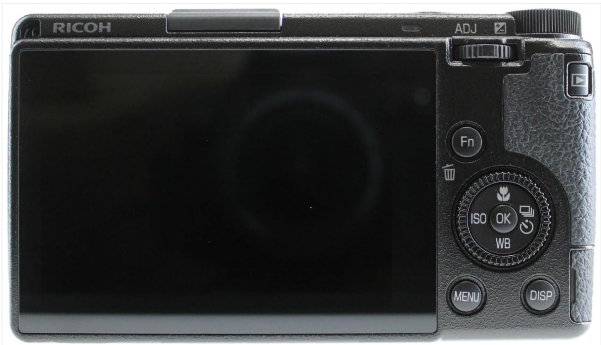
Figure 2: Back View. The rear of the camera shows the 3-inch touchscreen LCD. To the right, key controls include the ADJ dial, Fn (Function) button, Playback button, a four-way controller with ISO, OK, WB, and Flash/Drive Mode options, and the Menu and DISP (Display) buttons.
