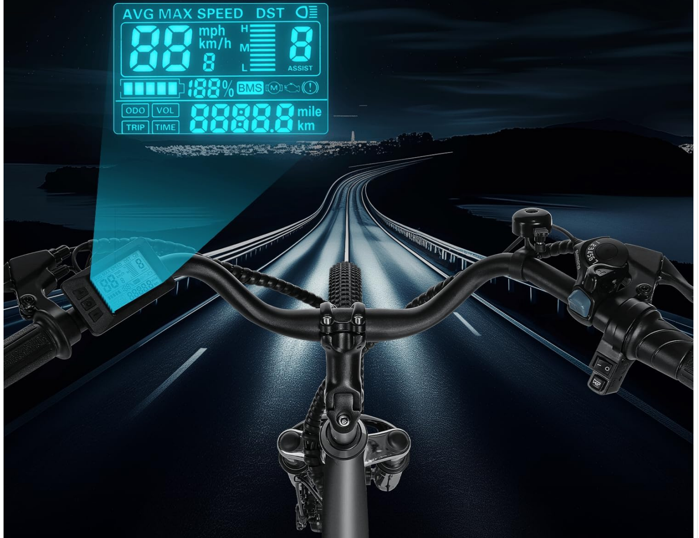
Figure 4: LCD Digital Display showing battery level, current speed, assist levels, mileage, and cruise control status.
