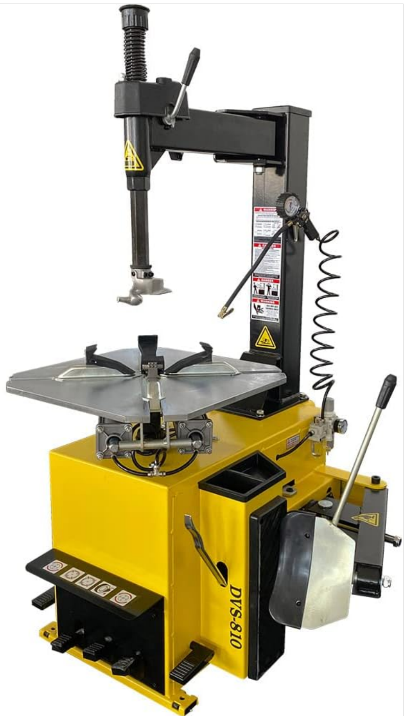
Figure 4: Advanced clamp positioning and foot-pedal controls for efficient tire changing.
