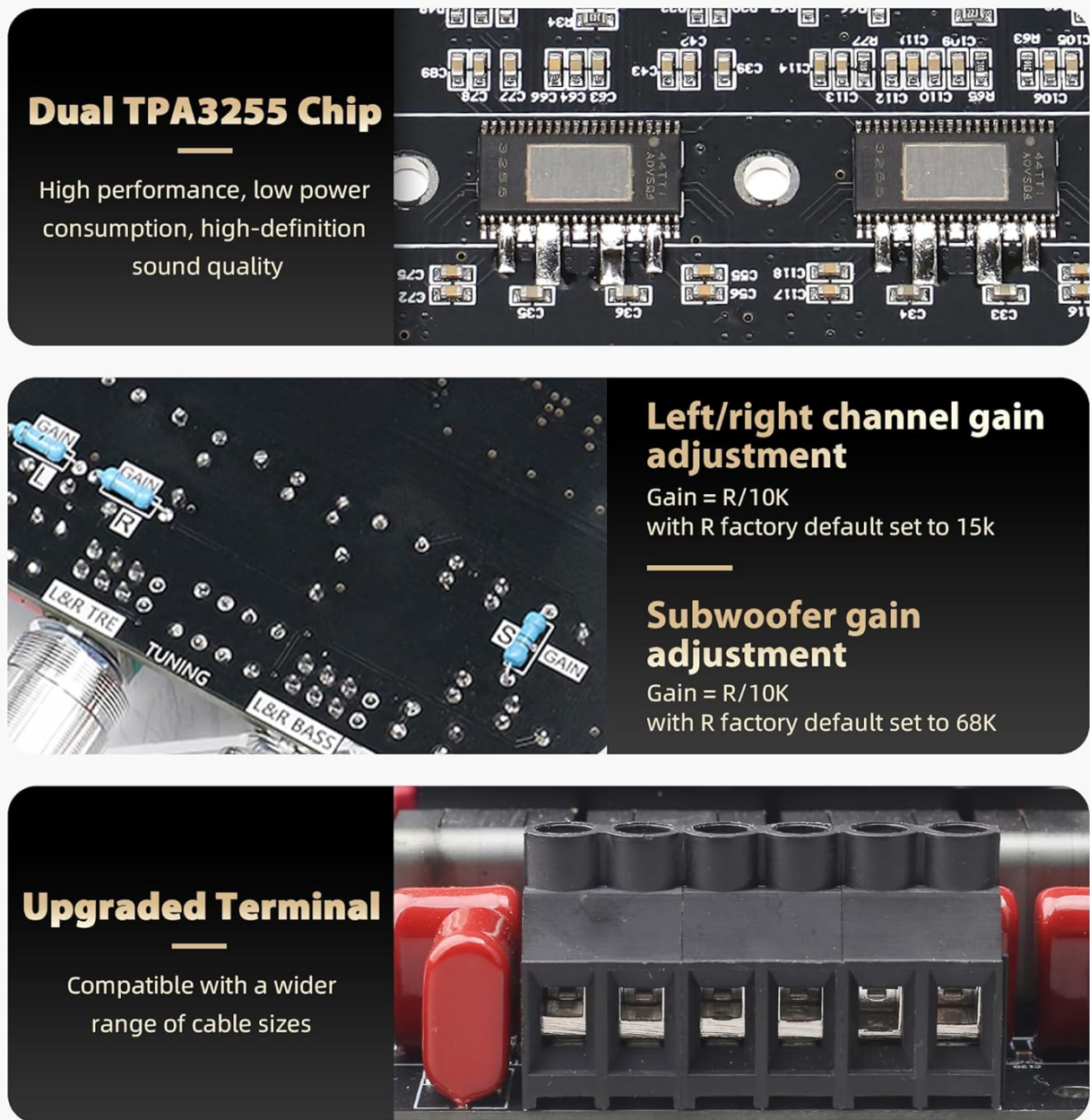
Figure 2: Dual TPA3255 Chip and Upgraded Terminal
