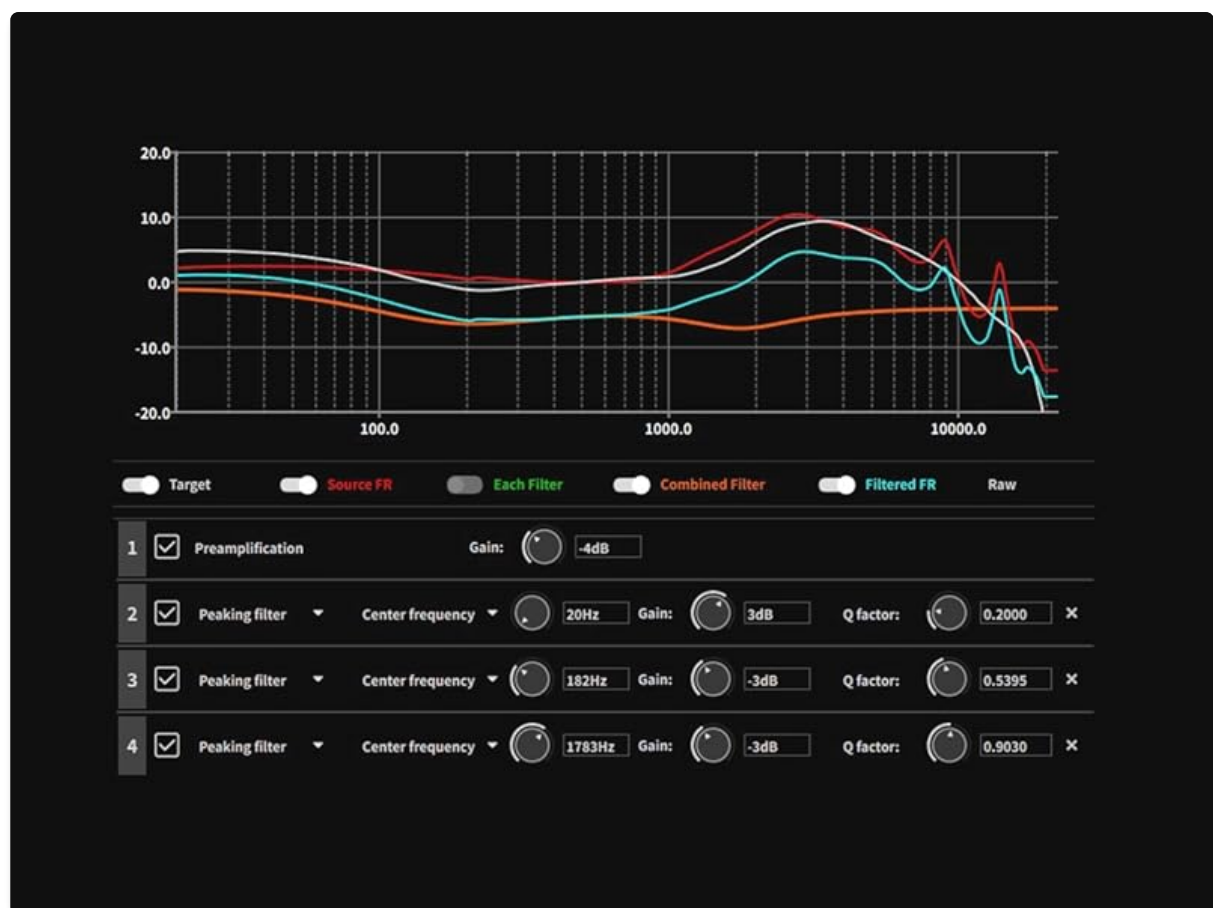
Figure 6: Software interface for precise PEQ adjustments, including target and filtered response curves.
