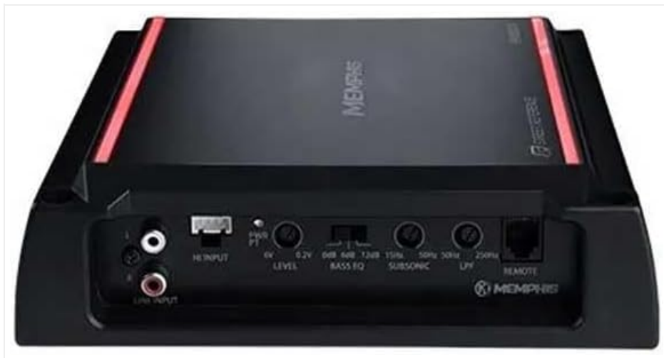
Image: Control panel of the SRX600.1V amplifier. This shows the various adjustment knobs and switches for tuning the audio output.
