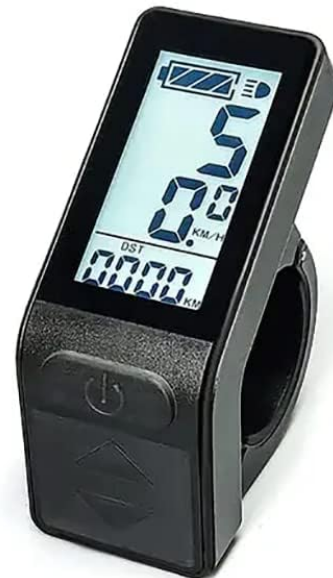
Figure 2.1: Compatibility verification. This image illustrates the necessity of matching the KT-LCD4 display with a KT (Kunteng) series controller for proper function. Users should check their controller for the 'KT' logo.
