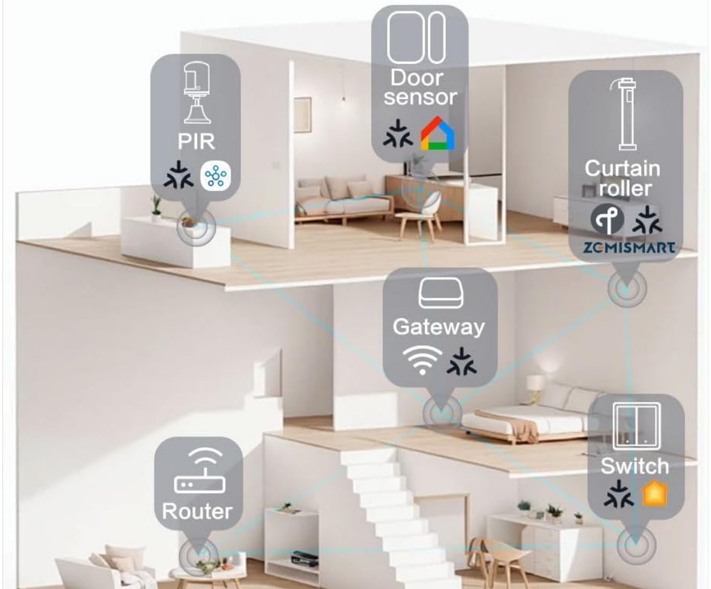
Image: A diagram depicting a multi-level smart home environment where various Matter devices, including the curtain roller, connect via a Thread mesh network, managed by a gateway and router.
