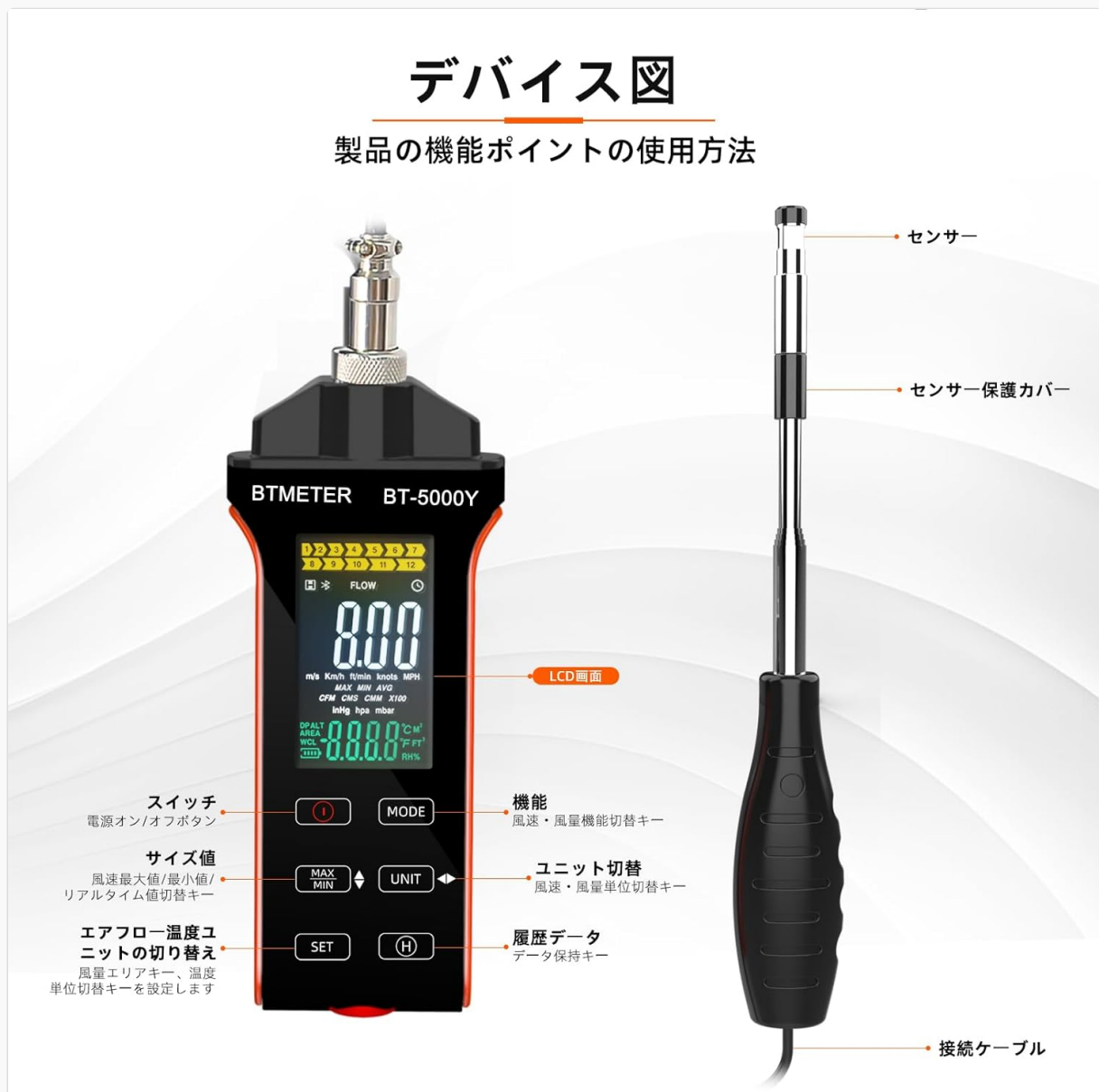
Figure 3.1: Device diagram illustrating key components and controls.
