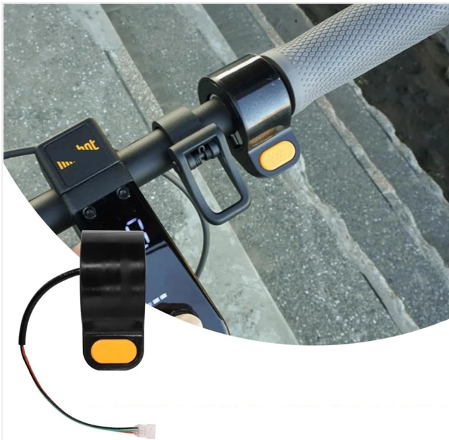
Image 5.5: The LHAQQ Thumb Throttle Assembly fully installed on a scooter handlebar, demonstrating its integrated appearance.
