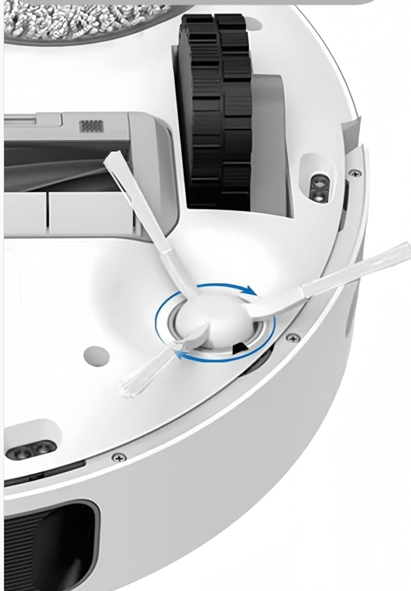
Figure 3: Nylon side brush designed for effective corner cleaning.
