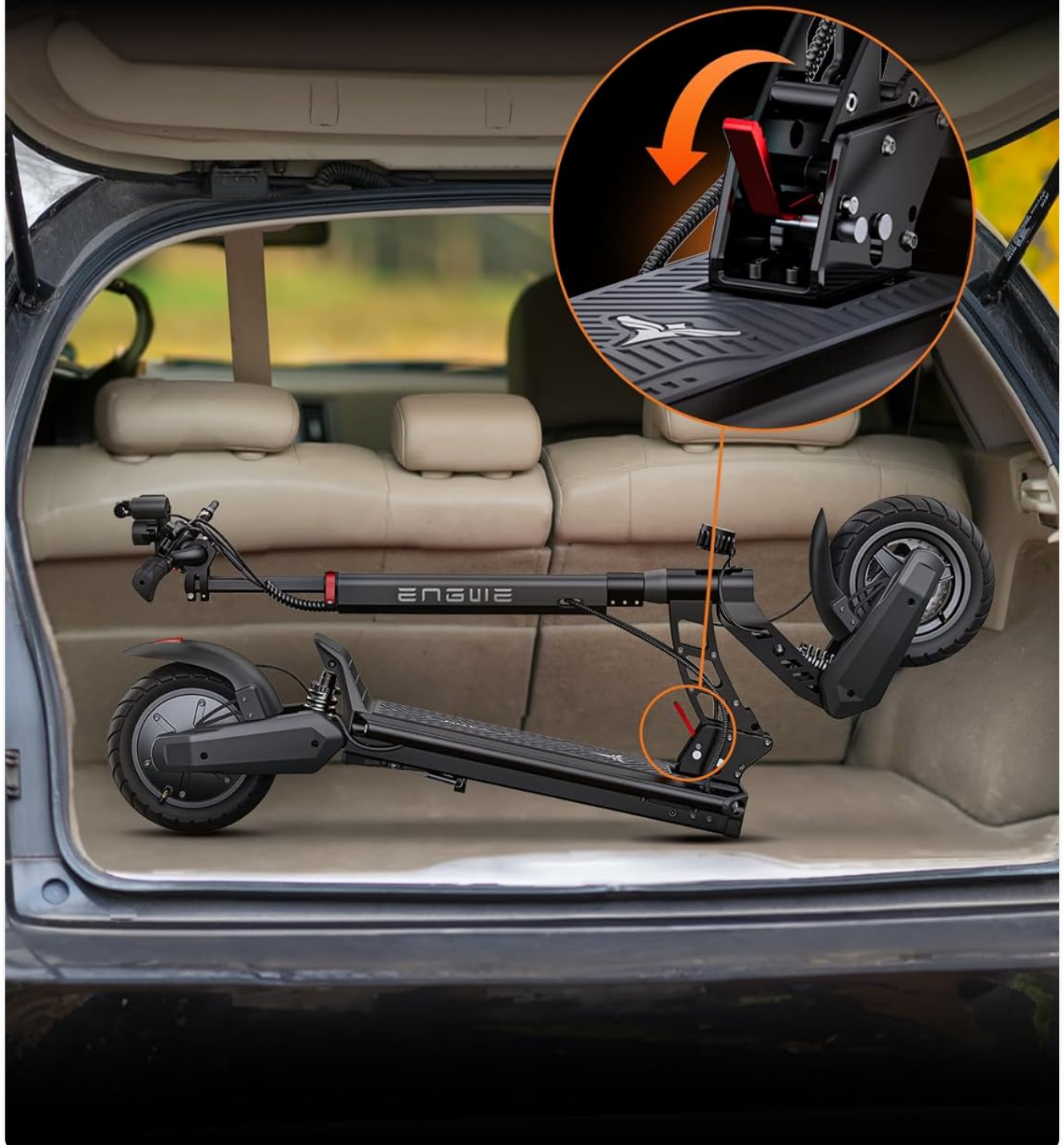
Figure 2: Portable Folding Design. The scooter folds for easy transport and storage.
