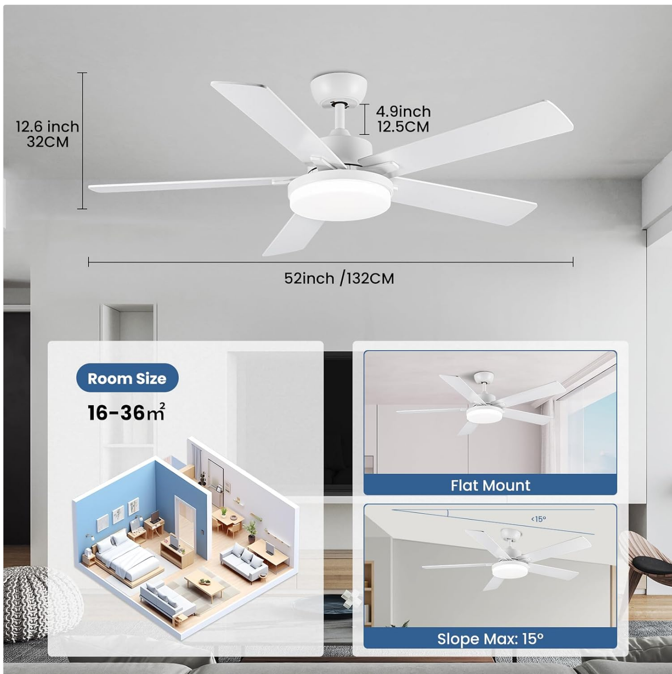
Image 4.1: Product dimensions (132cm diameter, 32cm height), recommended room size (16-36 m 2 ), and installation options for flat or sloped ceilings (max 15° incline).
