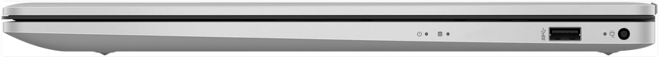
Image: Right side ports including a USB-A port and the power input.
