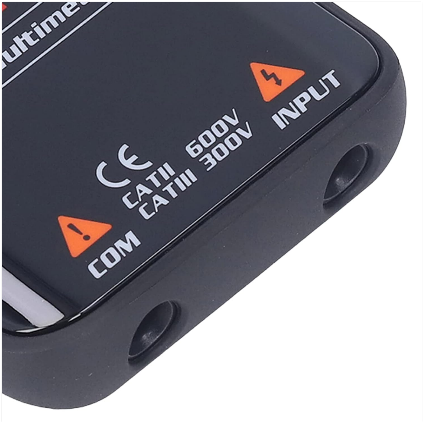
Figure 4.2: Input Jacks and Safety Markings.
