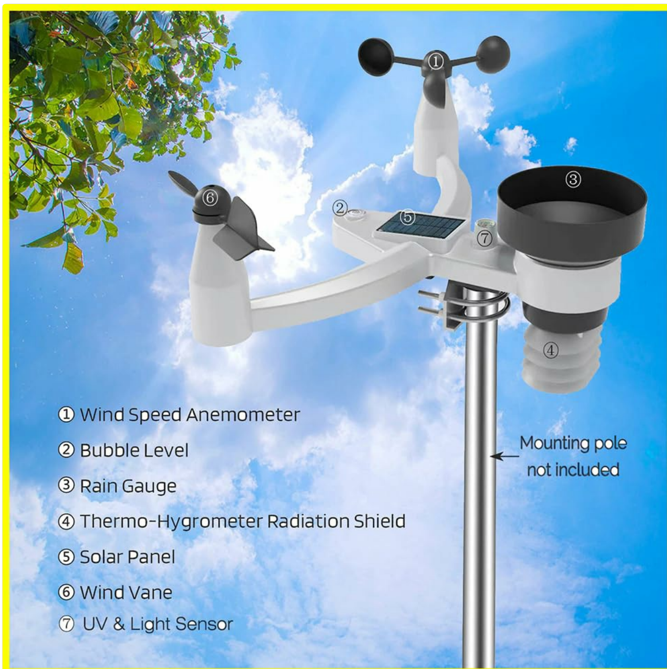
Figure 1: Integrated Outdoor Sensor Components.
