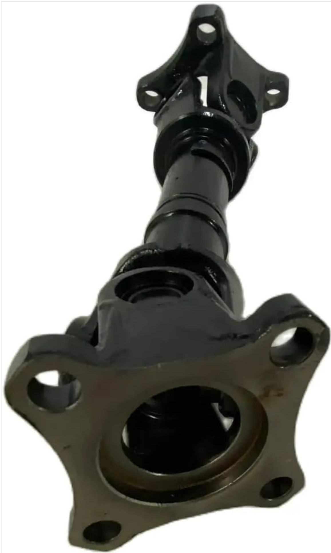
Figure 3.2: Angled view of the WKNYSYK Front Drive Shaft, highlighting the universal joints and mounting flanges. This perspective shows the detailed construction of the shaft's connection points.
