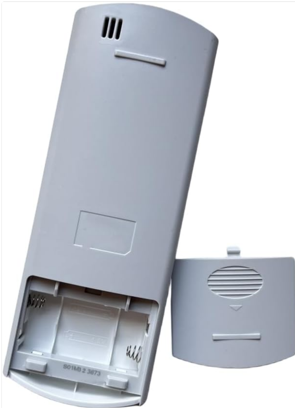
Figure 2: Rear view of the remote control with the battery cover removed, illustrating the battery insertion points.
