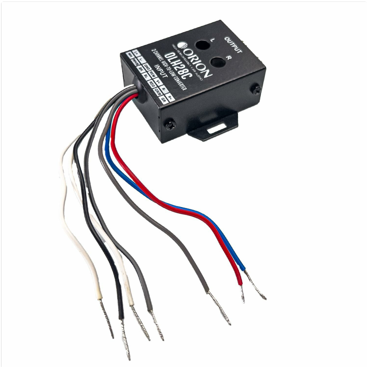
Figure 3.3: Angled view of the OLH28C, showing the complete set of input and output wiring for installation.
