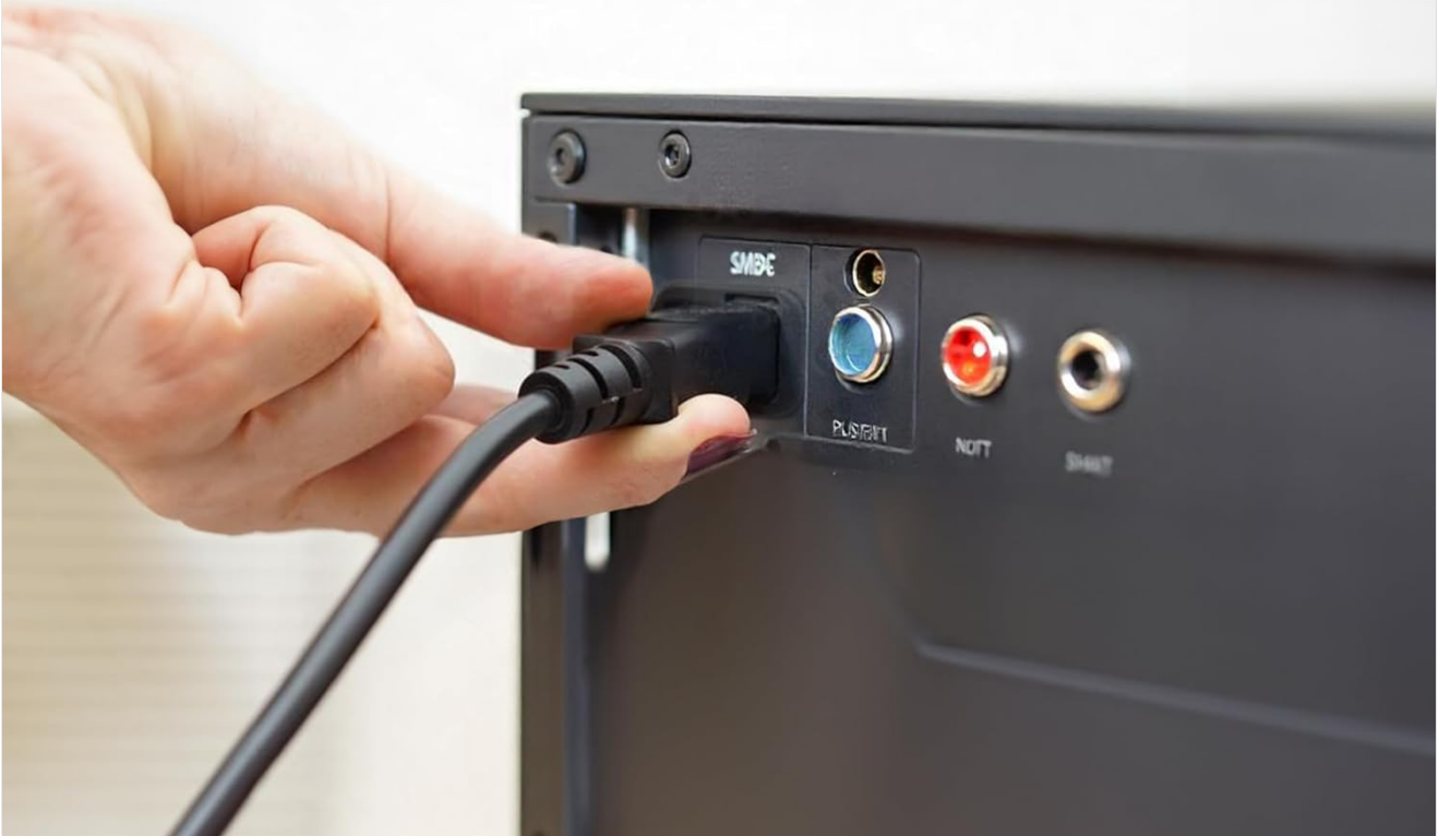
Figure 4: Visual guide for identifying the correct 3-pin power inlet (C13) compatible with this power cord.
