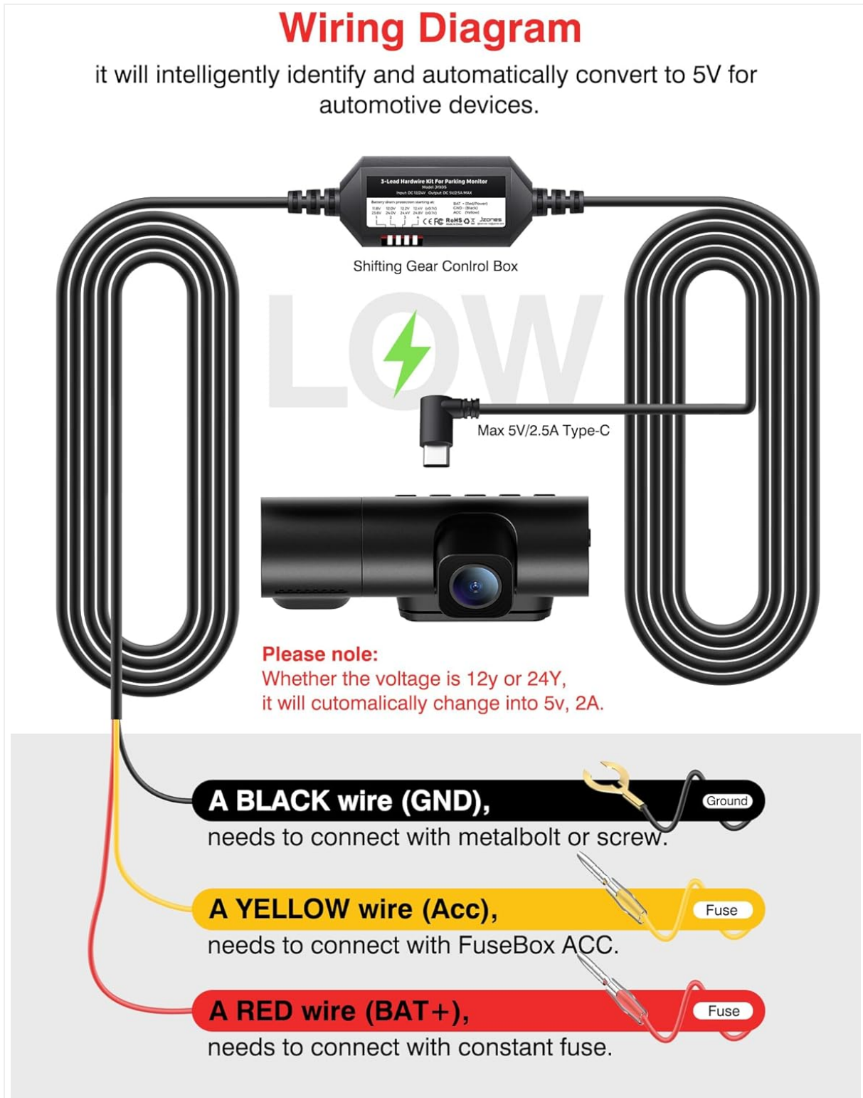
Figure 5.1: Detailed wiring diagram illustrating how to connect the hardwire kit's black, yellow, and red wires to the vehicle's electrical system.
