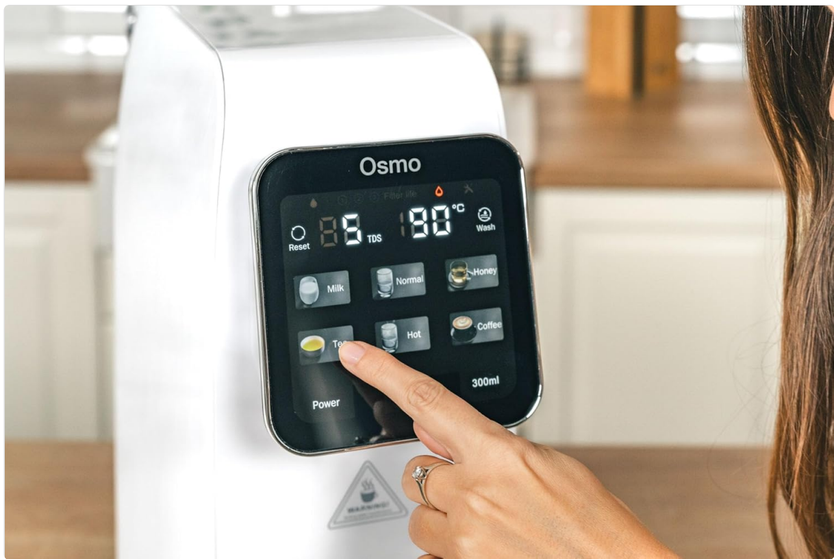
Figure 5.1: A user interacting with the touchscreen, selecting the 'Tea' preset temperature. The display shows current water quality (TDS) and temperature.
