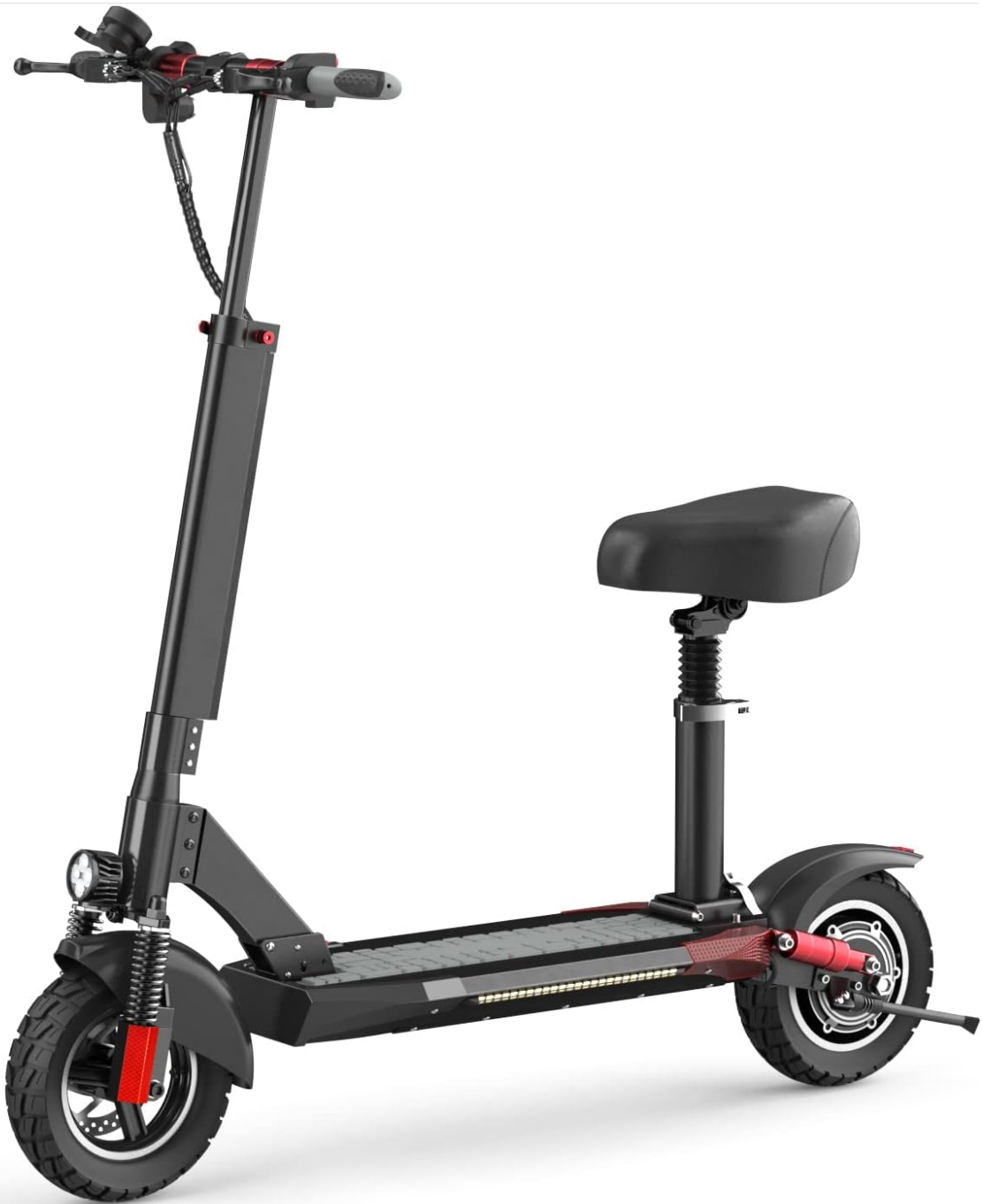
Image: A full view of the iENYRID M4 PRO S+1 Electric Scooter in black, featuring its 10-inch pneumatic tires, dual suspension, and detachable seat, highlighting its robust design.
