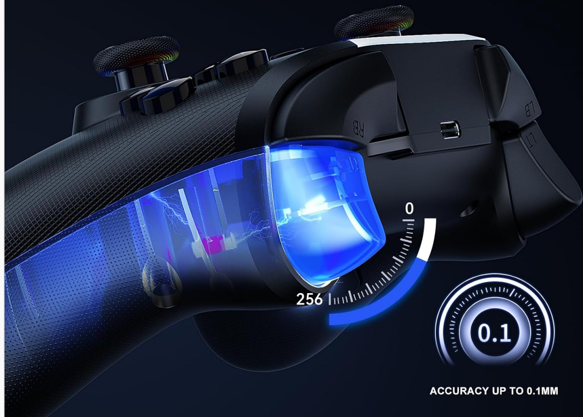
Image 3.2: Diagram showing the Hall Effect linear triggers, emphasizing precise control and smooth feeling with 0.1mm accuracy.
