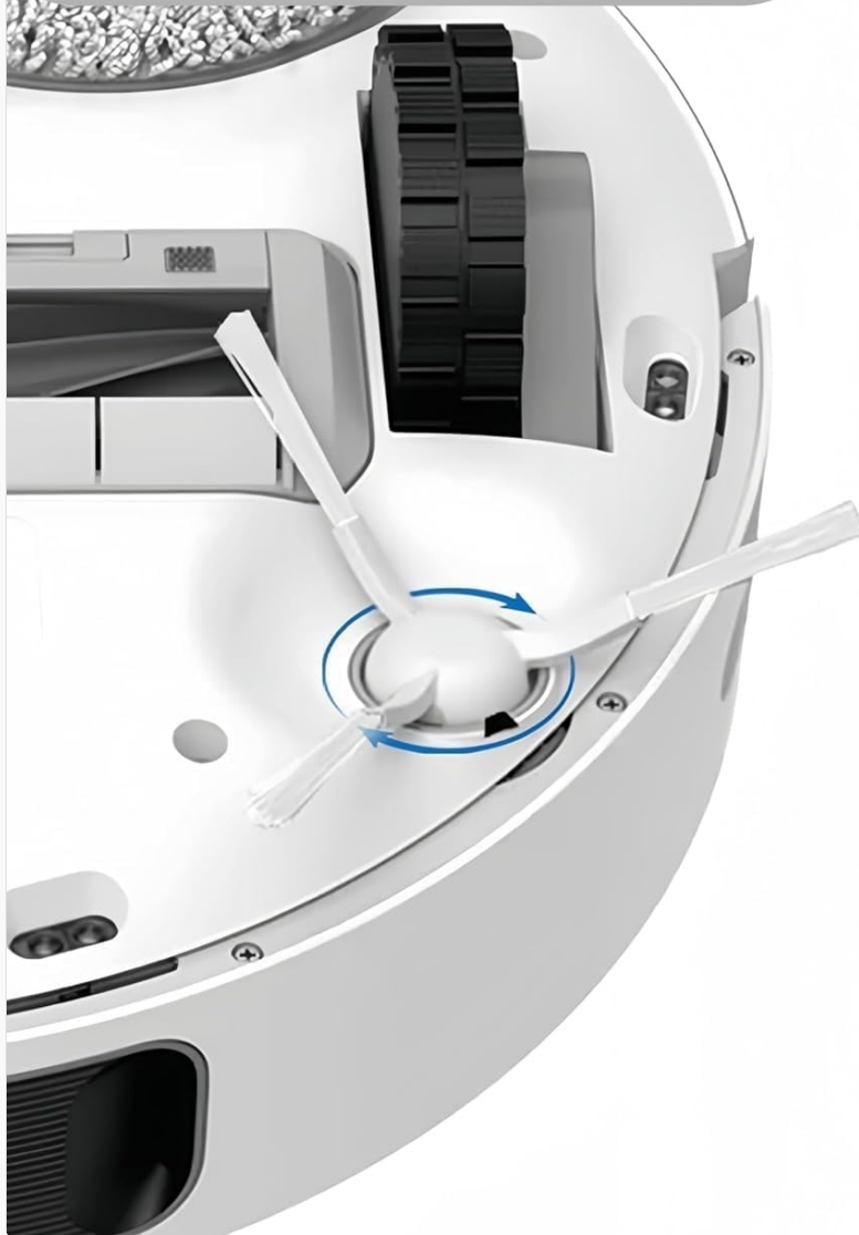
Image 2.3: The nylon bristle side brush, designed for thorough edge cleaning.
