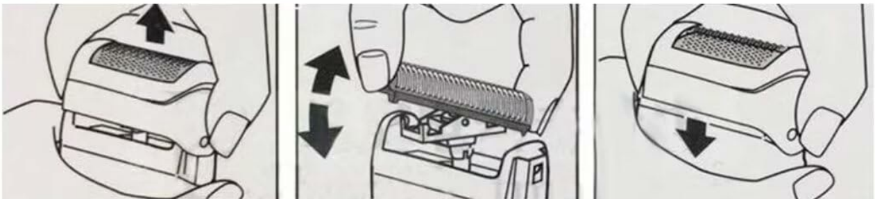
Figure 3: Visual guide for the replacement steps of the shaver foil and cutter.
