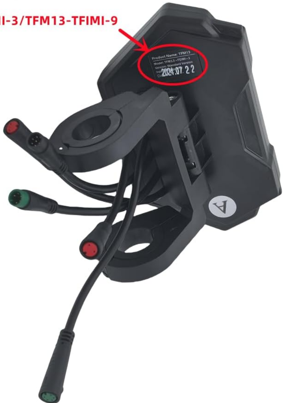
Figure 1.3: Rear view of the LCD Dashboard, displaying the product label. The label clearly indicates "Product Name: TFM13" and "Model: TFM13-TFIMI-3/TFM13-TFIMI-9", confirming the specific compatibility of this Model A display.
