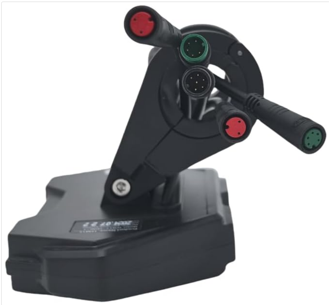
Figure 1.5: An alternative side view of the LCD Dashboard, providing a clearer look at the cable organization. This angle helps in understanding how the cables are routed and connected to the main unit.
