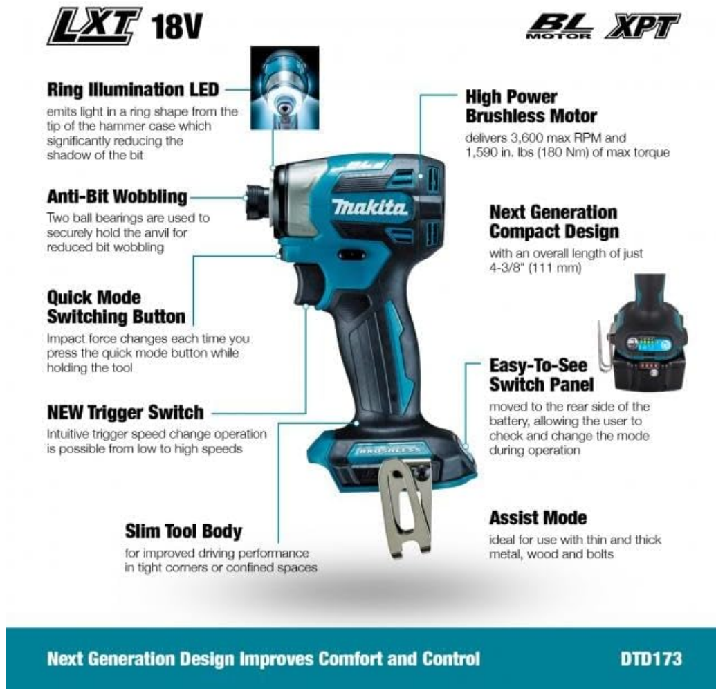
Figure 2: Detailed features of the Makita DTD173Z Impact Driver
