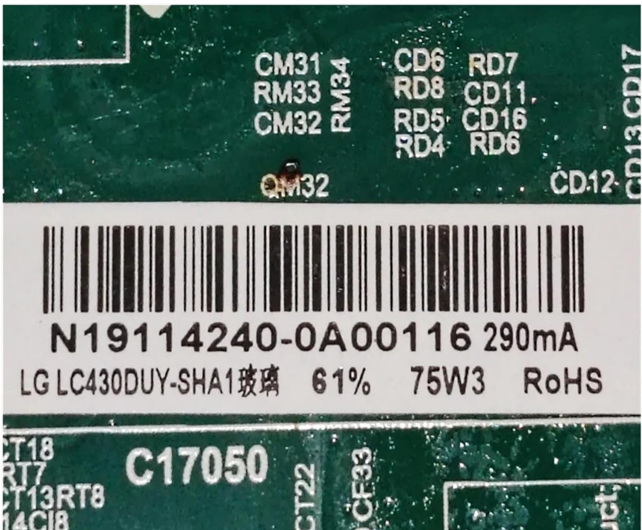
Figure 2: Label for White Transformer variant (N19114240-0A00116), 75W 290mA.
