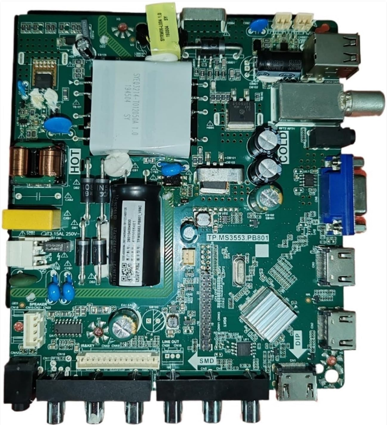
Figure 5: Overview of the motherboard showing various connection points.
