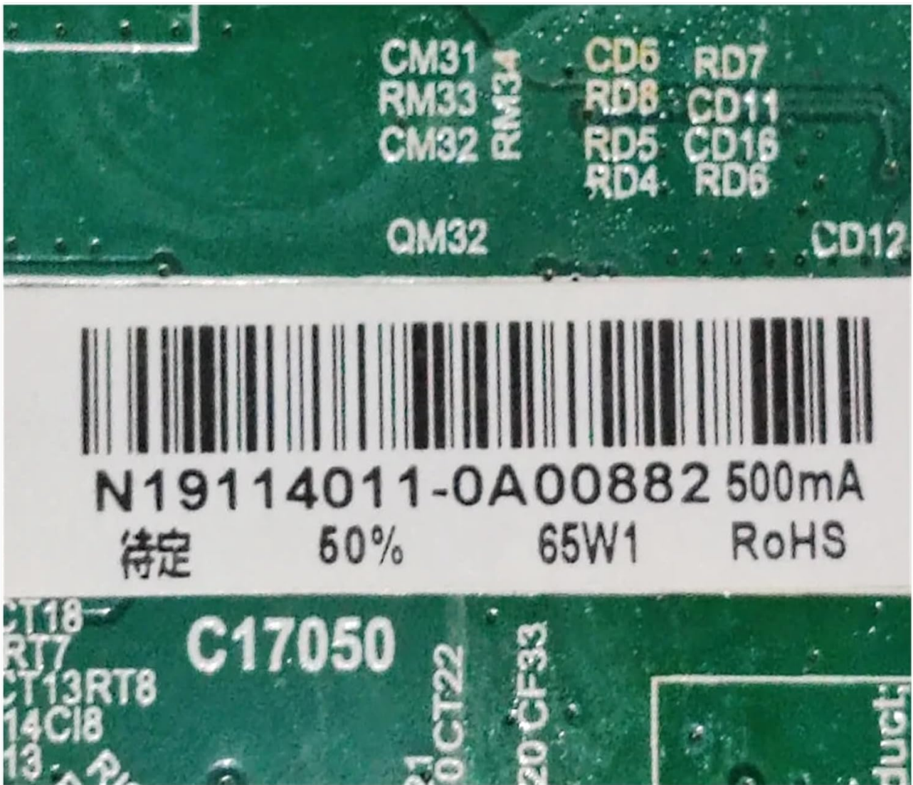
Figure 4: Label for Green Transformer variant (N19114011-0A00882), 65W 500mA.
