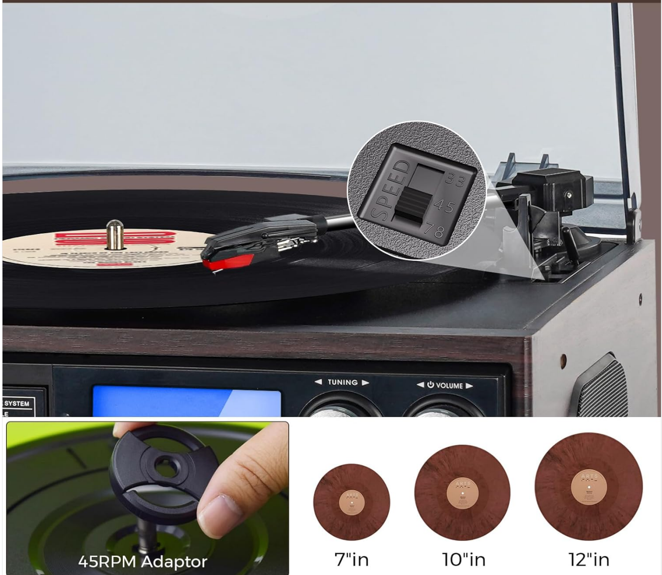
Figure 6.1: Turntable Speed Selection and 45 RPM Adapter. This image shows the speed selector switch (33, 45, 78 RPM) and the 45 RPM adapter for playing records with larger center holes.
