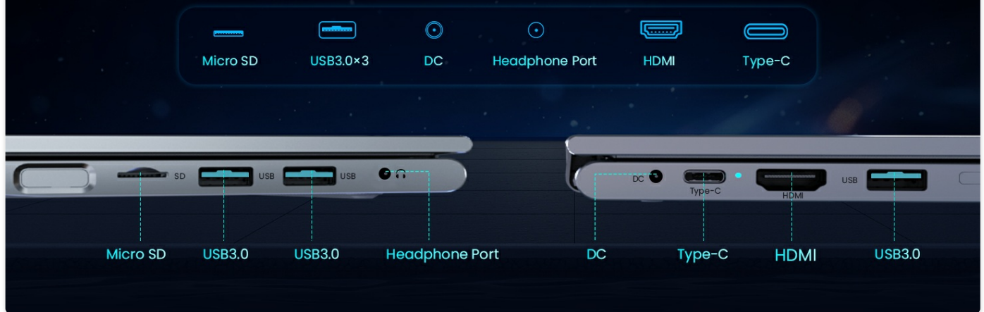
Image: Detailed view of the laptop's various ports, including Micro SD, USB 3.0, Headphone, HDMI, and Type-C.
