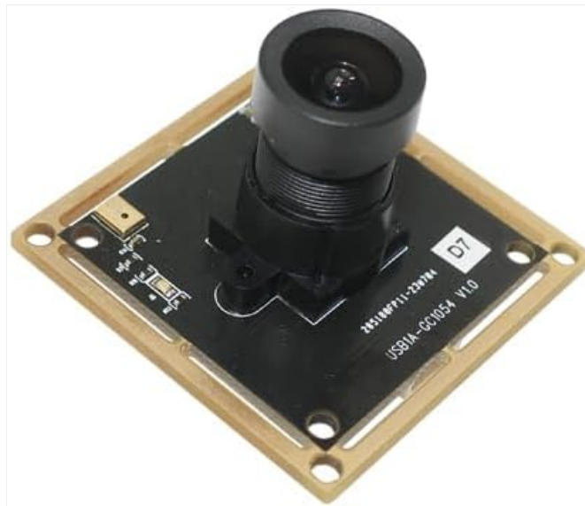
Image: Angled view of the YDS-USB1A-GC1054 V1.0 USB camera module, showing the lens and the square PCB with mounting holes.
