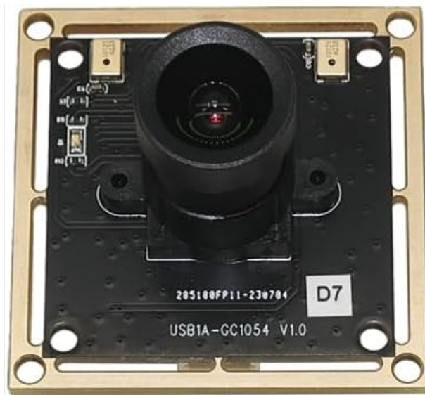
Image: Top view of the YDS-USB1A-GC1054 V1.0 USB camera module, showing the lens and the main components on the PCB.
